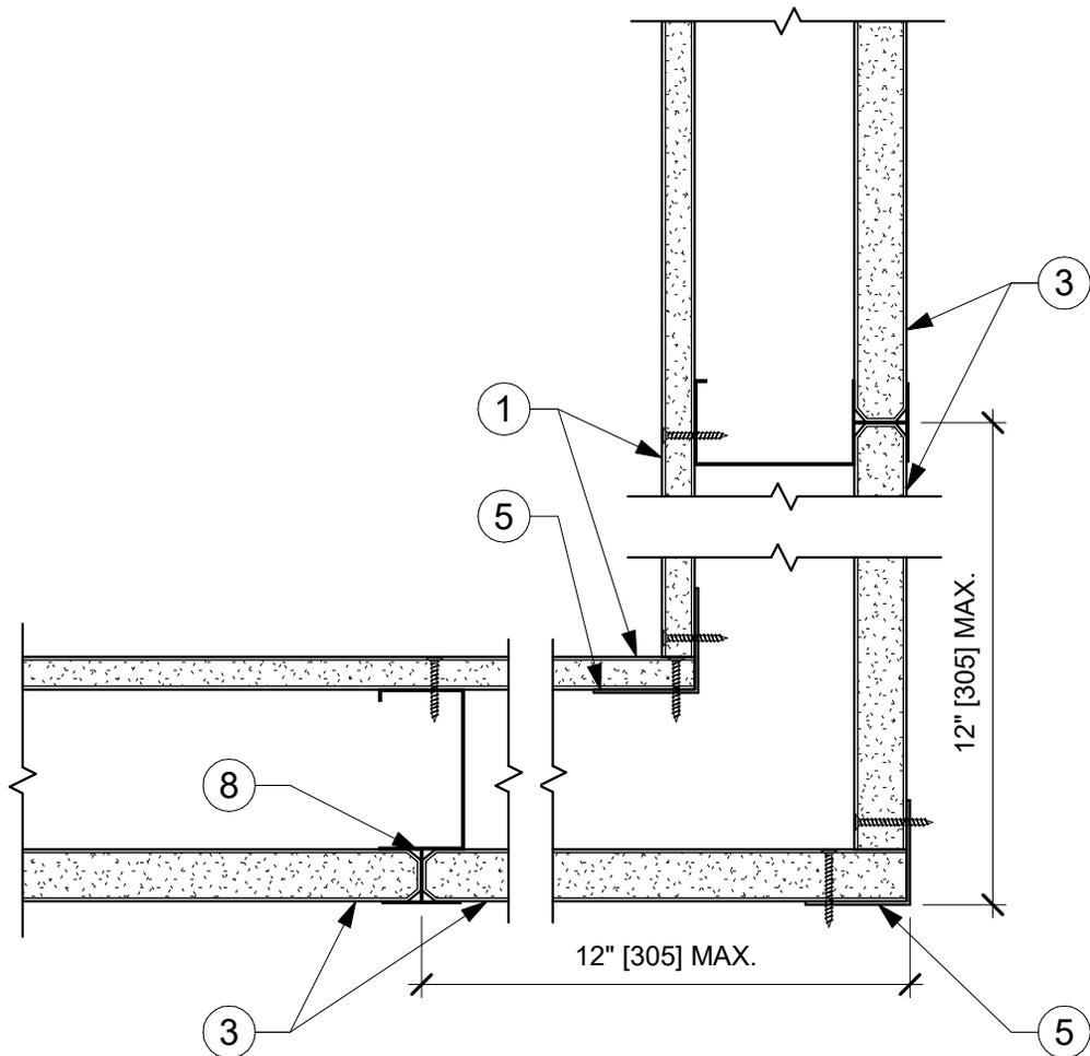
**1-HOUR SHAFTWALL CORNER DETAIL**
