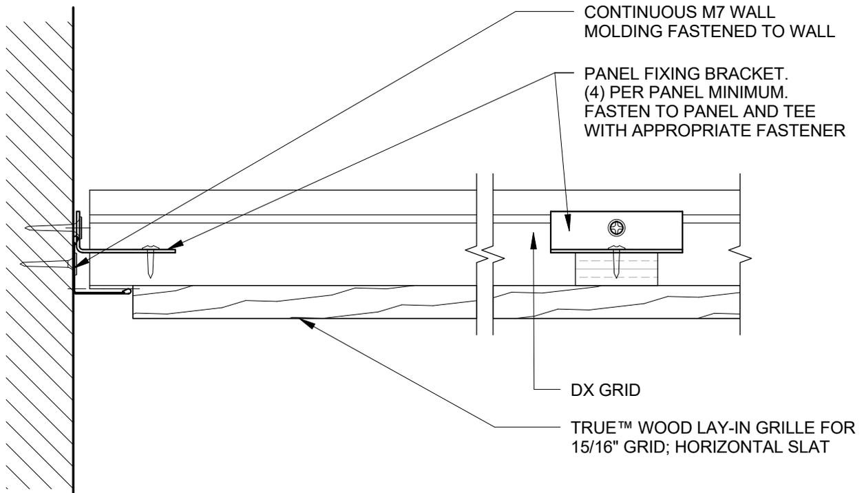
NOTE: PROVIDE PANEL FIXING BRACKETS AT PERIMETER, WHEN PANELS DO NOT ENGAGE ON ALL 4 SIDES WITH GRID OR WHEN PANELS ARE MODIFIED IN ANY WAY
