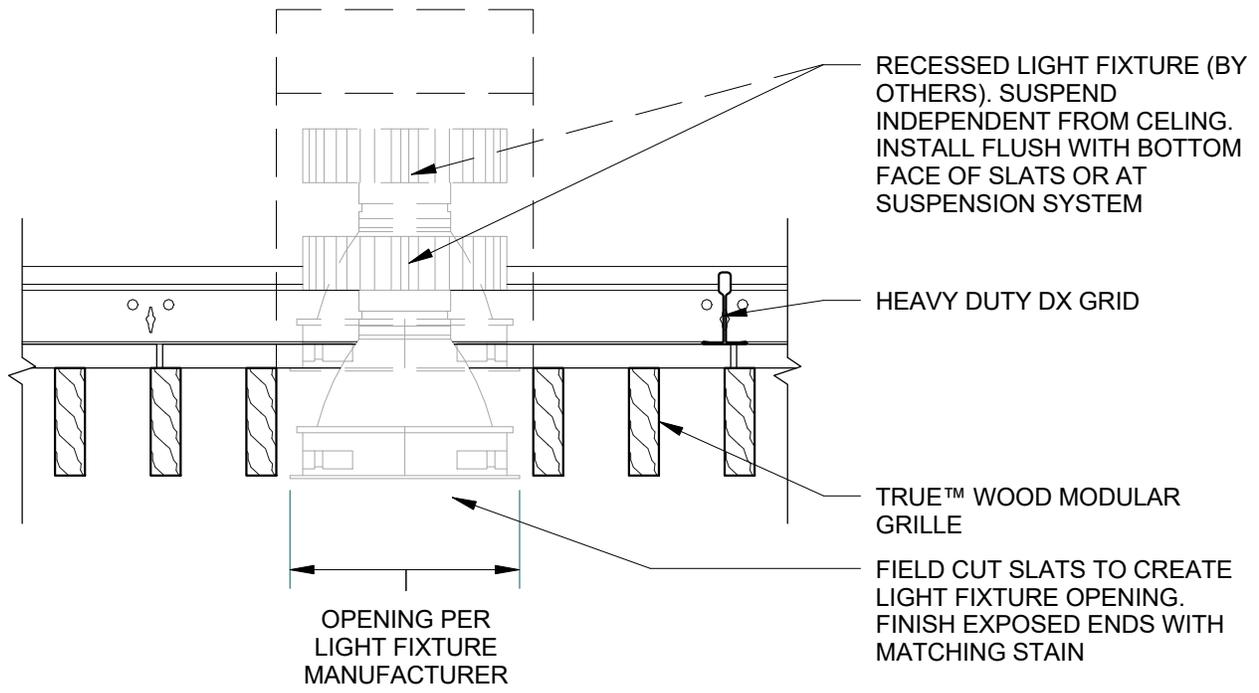
RECESSED LIGHT FIXTURE (BY OTHERS). SUSPEND INDEPENDENT FROM CEILING. INSTALL FLUSH WITH BOTTOM FACE OF SLATS OR AT SUSPENSION SYSTEM
