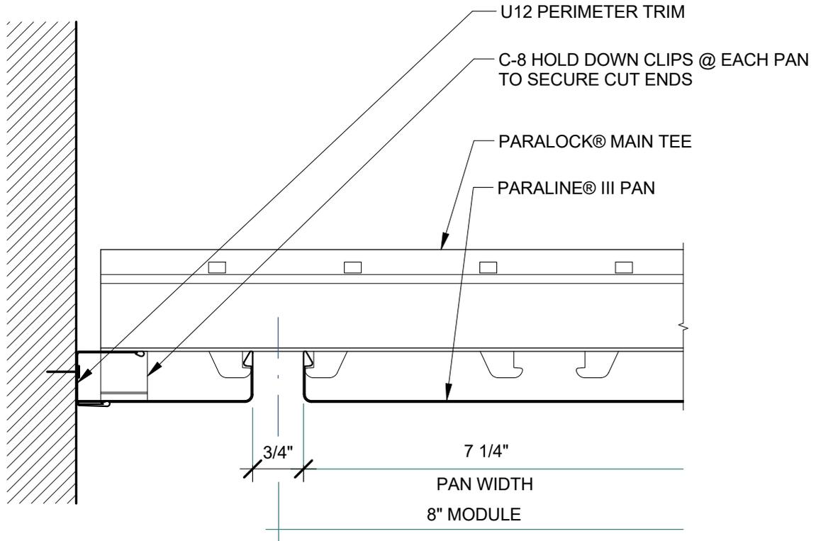
PARALINE® III: OFF-MODULE PANEL AT MAIN TEE - U12 MOLDING
