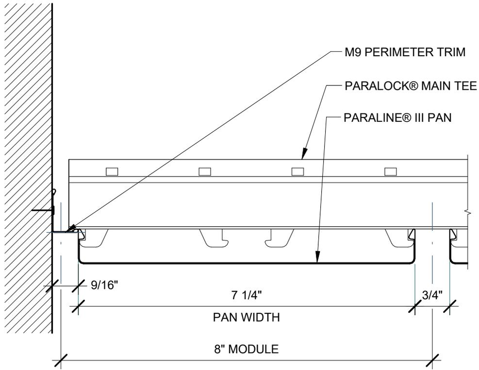
PARALINE® III: ON-MODULE PANEL AT MAIN TEE - M9 MOLDING
