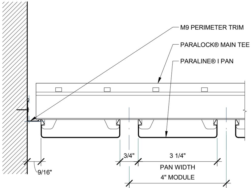
PARALINE® I: ON-MODULE PANEL AT MAIN TEE - M9 MOLDING
