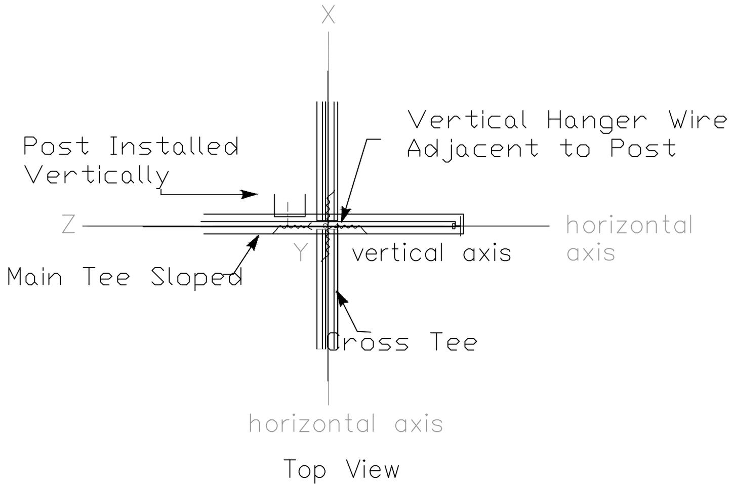
Hanger Wire—Horizontal Axis Top View
