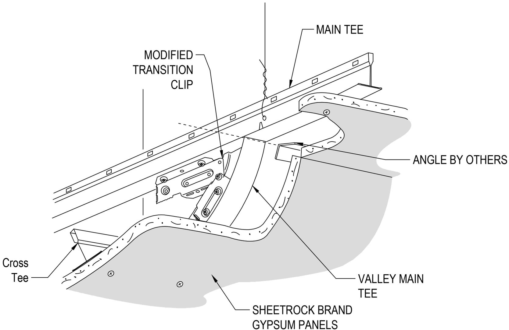
Curved Soffit to Boxed Soffit
