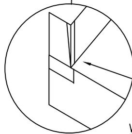
20 MIL ELASTOMERIC SHEET MEMBRANE. CUT & PATCH AT CORNER. SEAM WITH SOLVENT WELDING OR THERMAL WELDING.
