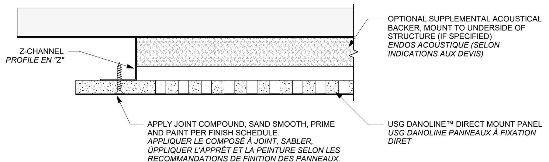
USG DANOLINE™ DIRECT MOUNT PANEL WITH Z-FURRING CHANNELS
