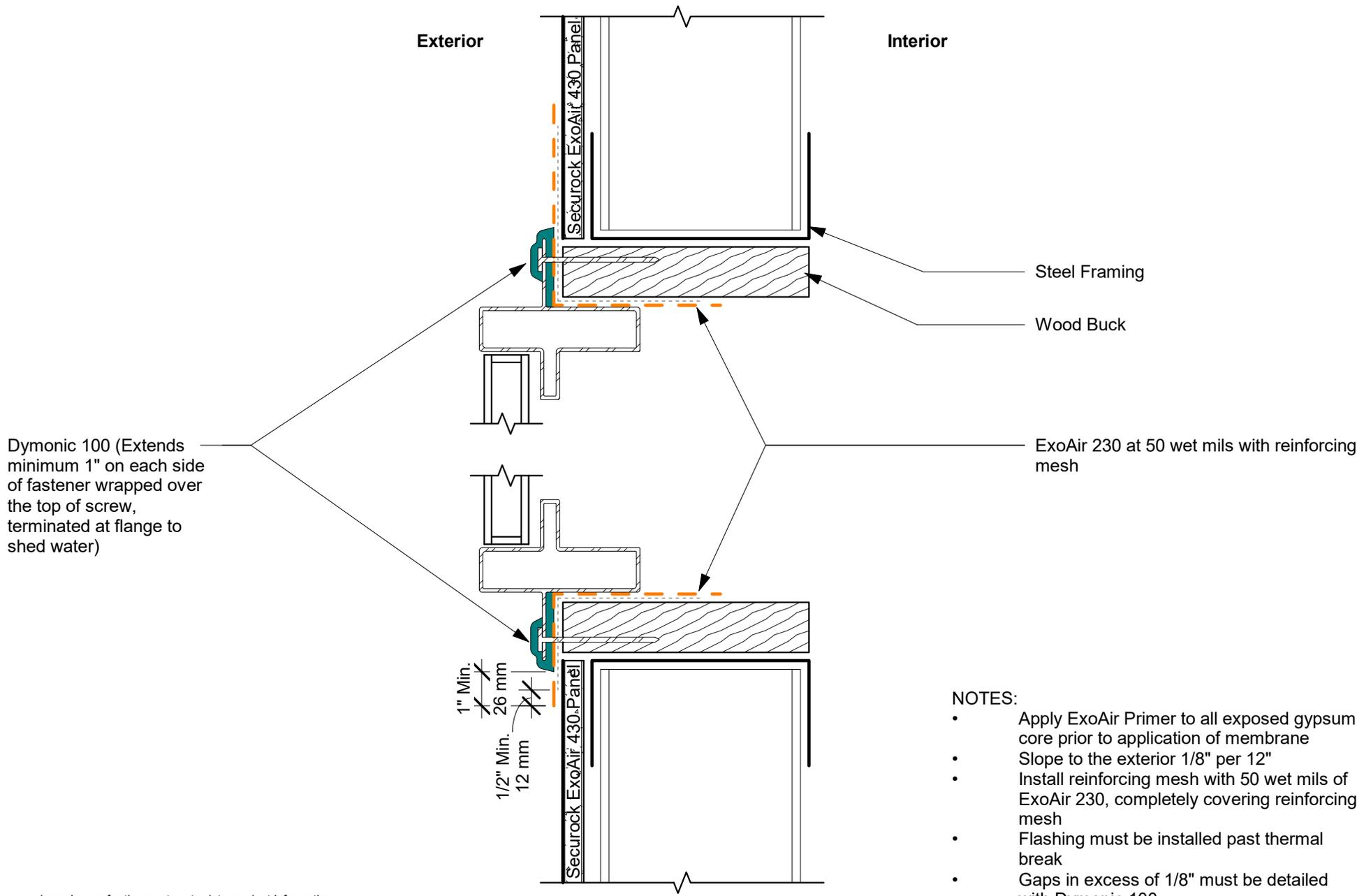
Dymonic 100 (Extends minimum 1" on each side of fastener wrapped over the top of screw, terminated at flange to shed water)
