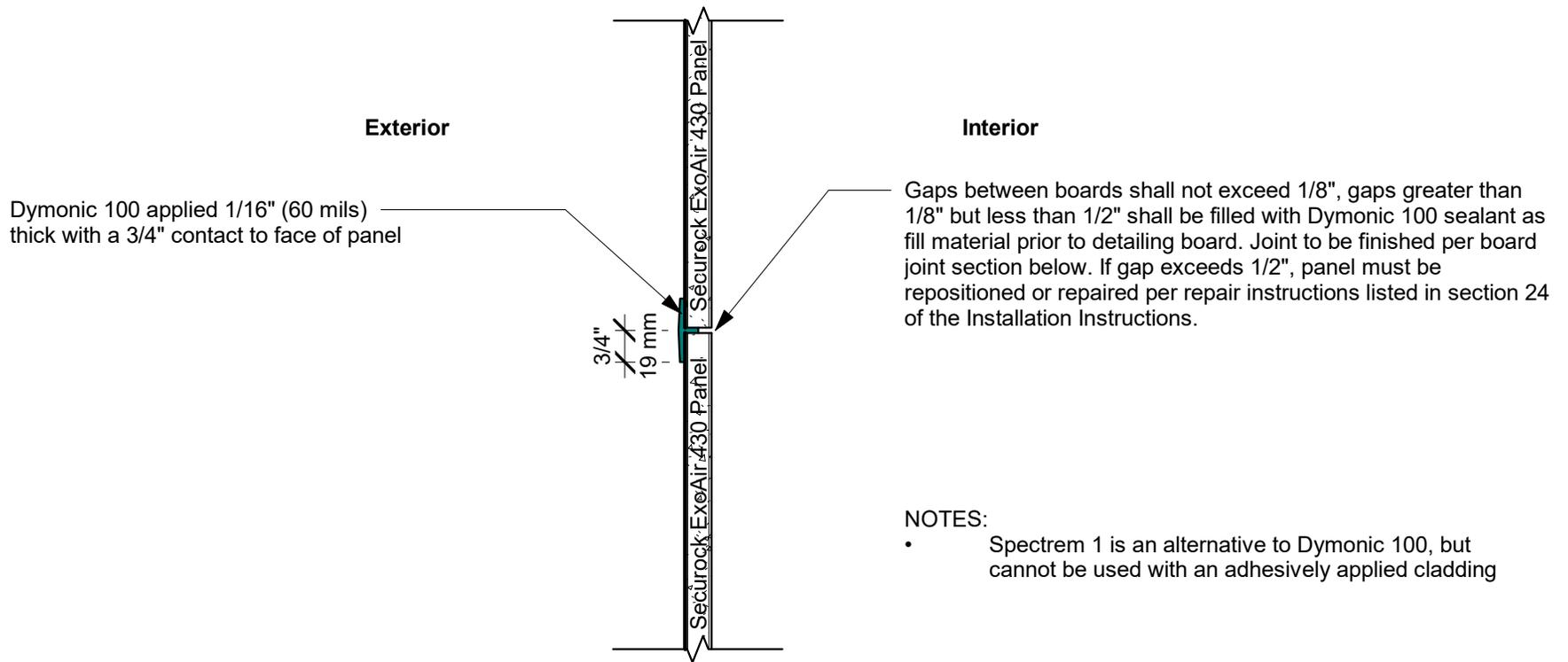
Dymonic 100 applied 1/16" (60 mils) thick with a 3/4" contact to face of panel
