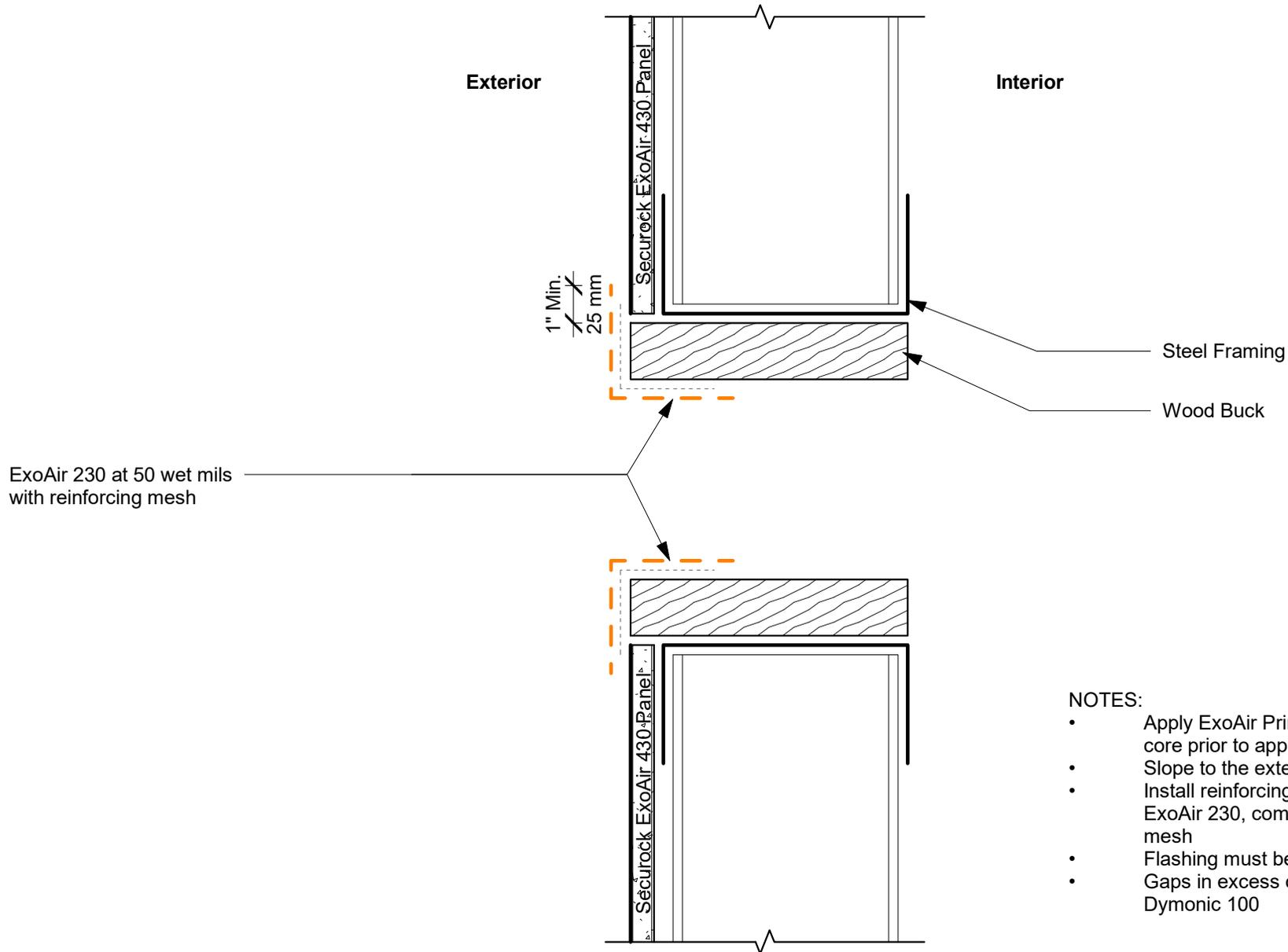
ExoAir 230 at 50 wet mils with reinforcing mesh
